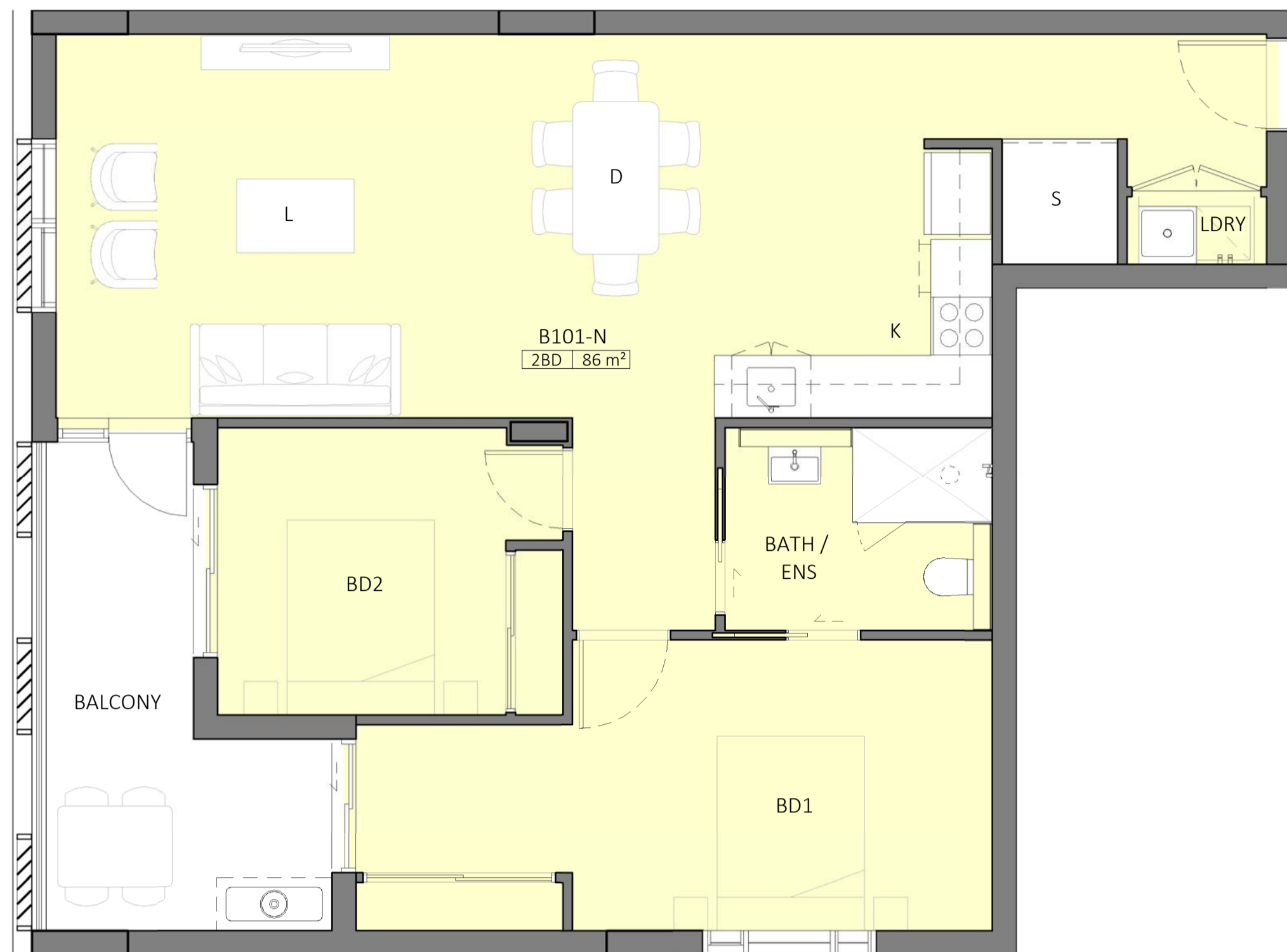
1 ADAPTABLE UNIT TYPE N - PRE DA-0-113 1:50 NO. OF UNITS - (10) - B101, B107, B201, B207, B301, B307, B401, B407, B501, B507
